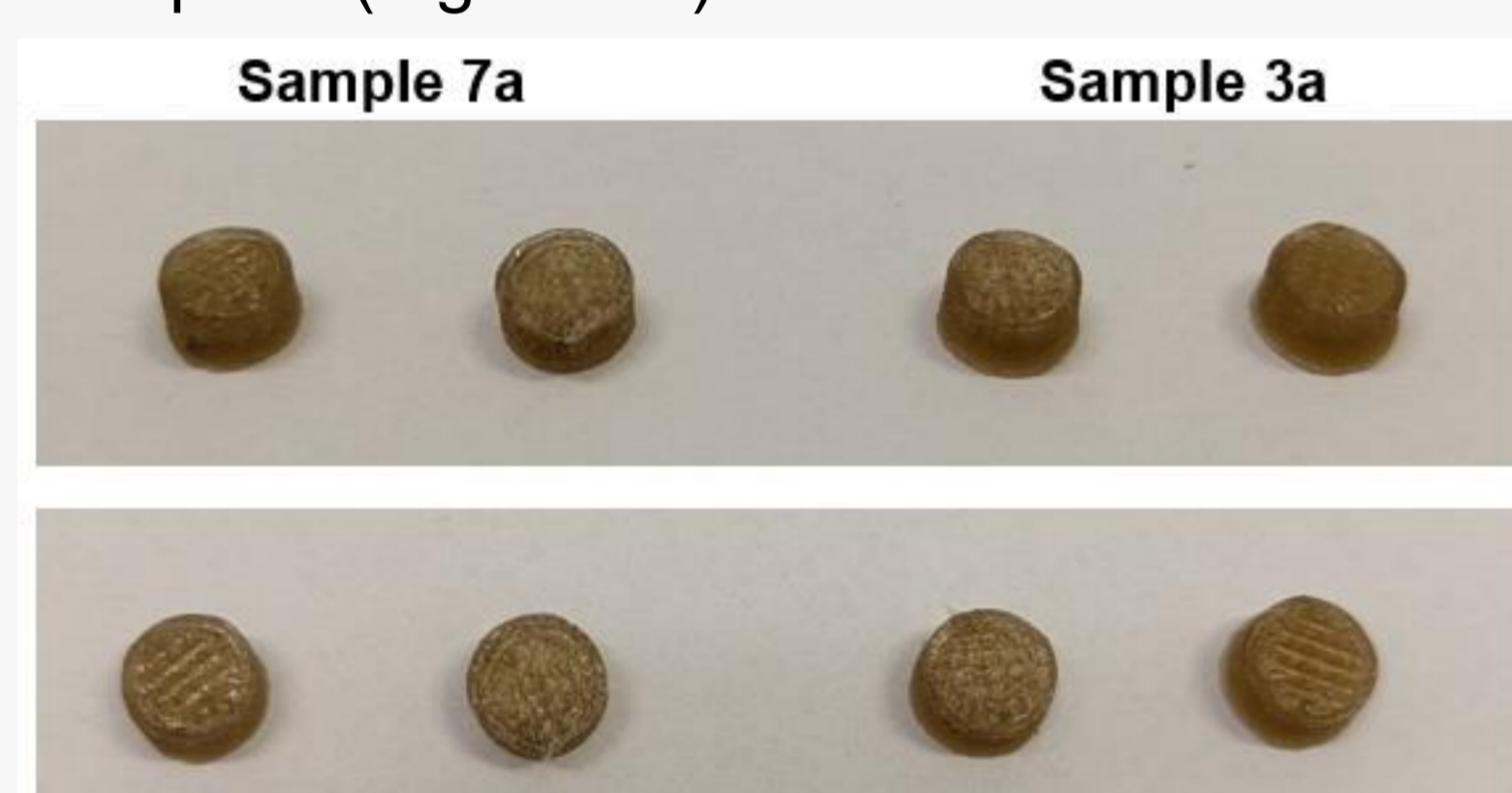
Figure 1: METT images of FF and NIF ASD-discs with different polymers and drug loads in 0.3 ml phosphate buffer (pH 6.8). Erosion time 60 min.
